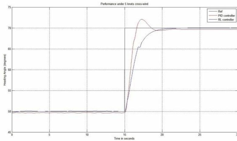
Figure 4: 5 knots wind disturbance
