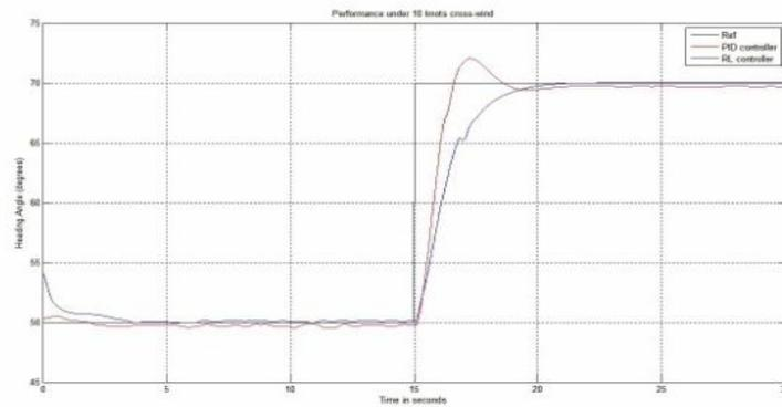
Figure 5: 10knots wind disturbance
