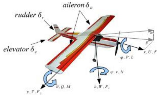
**Figure 1:** UAV Control surfaces
