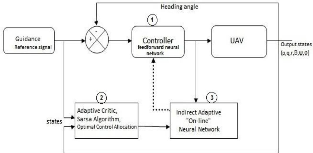
**Figure 3: Experiment Block Diagram**
